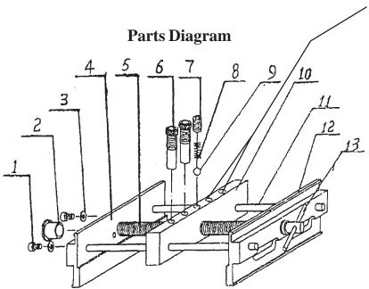
**Note:** There are 4 holes along the top of the Jig. Only 2 of the holes accept threaded bushings. The other 2 holes accept 7/16" and 1/2" drill bits.
